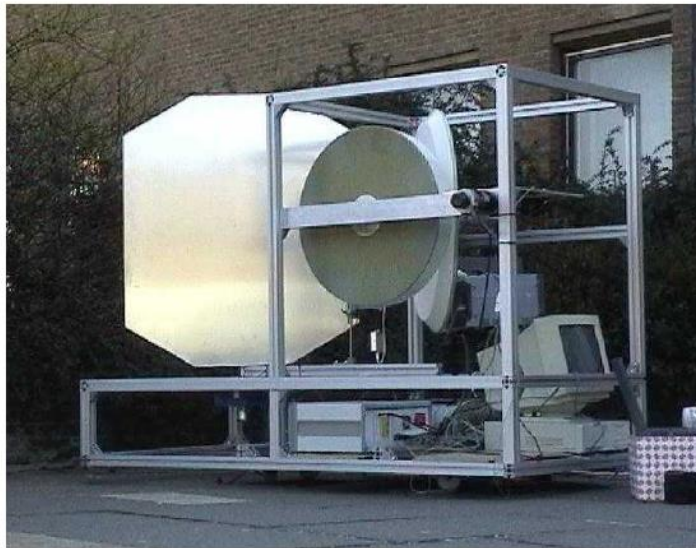
Figure 4.24. NASA double-disc imager showing spherical and plane mirrors
